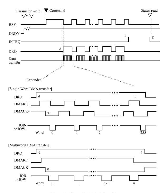
Figure 5.7 Normal DMA data transfer
